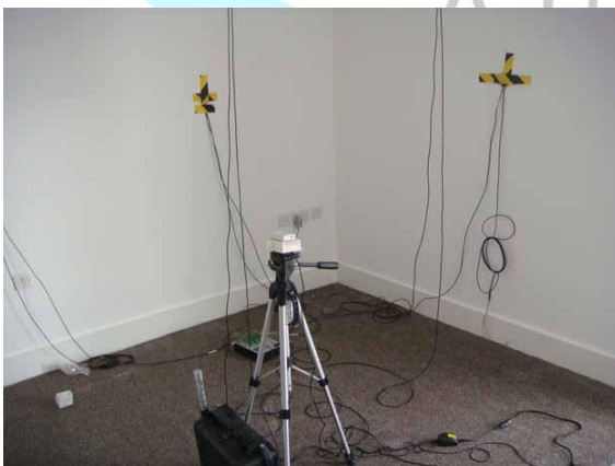
Figure 2: Heat flux sensors; photograph courtesy University College London
