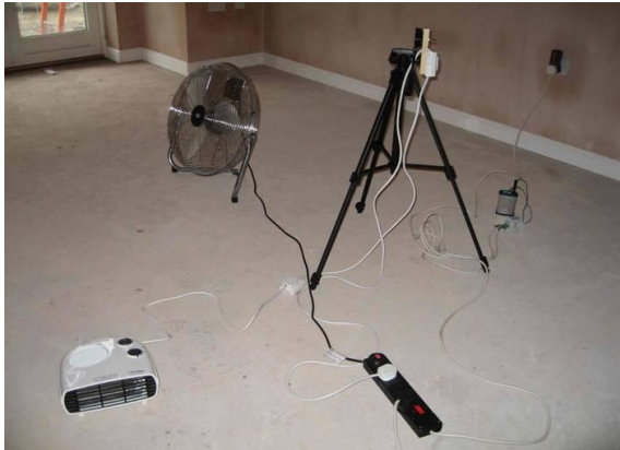
Figure 1: Co-heating test equipment; photograph courtesy Leeds Metropolitan University
